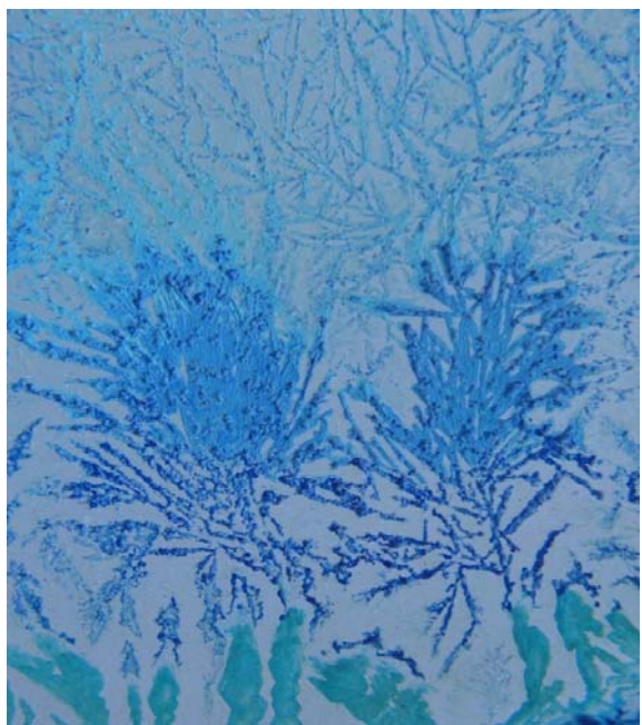
Fig. 6. Crystals formed after drying of an aqueous solution of CuCl 2 , previously exposed to low-frequency (0÷100 Hz) EMFs. For contrast, the crystals formed were treated with ammonia vapors.
