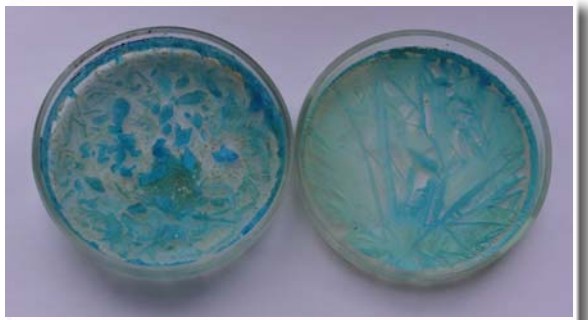
Fig. 2. It is the crystals that formed after the drying of solutions of \text{CuSO}_4 prepared on water potentials of +250 mV (left) and -250 mV (right).
