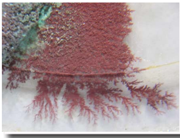
Fig. 5. It is a copper powder located near the boundary of waters with positive (above the line) and negative (below the line) potentials [2, 3].
