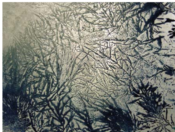
Fig. 7. Crystals formed after drying of an aqueous solution of CuCl 2 , in which was previously a direct current.
