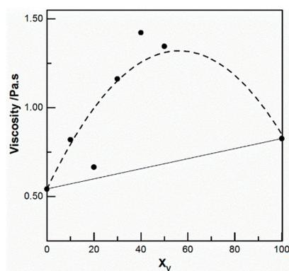
**Figure 1.** Variation of the viscosity of chitosan CS-102/ PEO ( $M = 1000 \text{ kg/mol}$ ) mixtures in 0.5 M acetic acid at  $0.5 \text{ s}^{-1}$  as a function of weight fraction of PEO ( $X_v$ ). Total polymer concentration 5%  $w/v$ . PEO: poly(ethylene oxide); CS: Chitosan.
