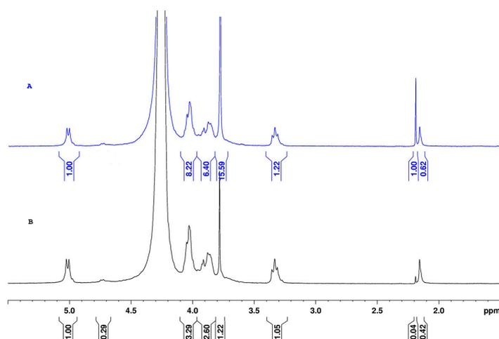
**Figure 6.** As spun fibers from the mixture CS/PEO (80/20) dissolved in acidic  $\text{D}_2\text{O}$  (A); Stabilized and washed chitosan fibers from the mixture CS-102/PEO 80/20 dissolved in acidic  $\text{D}_2\text{O}$  (B).
