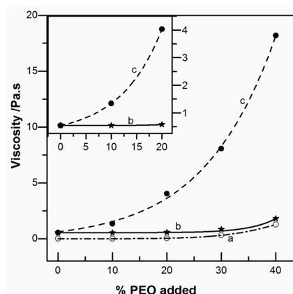
**Figure 2.** Variation of the viscosity at  $0.5 \text{ s}^{-1}$  of added PEO ( $M = 1000 \text{ kg/mol}$ ) expressed in percent of total polymer concentration in the mixtures. (a) PEO solution in 0.5 M acetic acid  $\circ$ ; (b) additivity calculated for each values of “a” added into pure chitosan CS-102  $\star$  and (c) blends chitosan CS-102/PEO as a function of the weight fraction of PEO  $\bullet$ .
