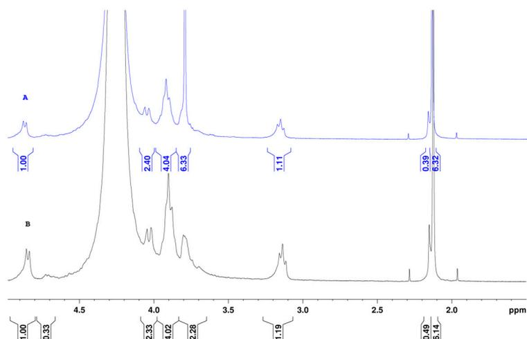
**Figure 5.**  $^1\text{H}$ -NMR spectrum for the CS-102/PEO (80/20) mixture solubilized in 0.5 M acetic acid with added  $\text{D}_2\text{O}$  (A) and CS-102 solubilized in 0.5 M acetic acid with added  $\text{D}_2\text{O}$  (B).
