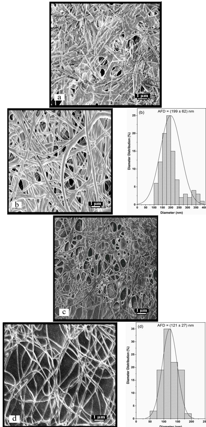
**Figure 4.** The SEM images of the membrane surface of chitosan/PEO at different ratios. (a) 60/40 neutralized in water; (b) 60/40 neutralized in ethanol/water mixture; (c) 80/20 neutralized in water; and (d) 80/20 neutralized in ethanol/water mixture.
