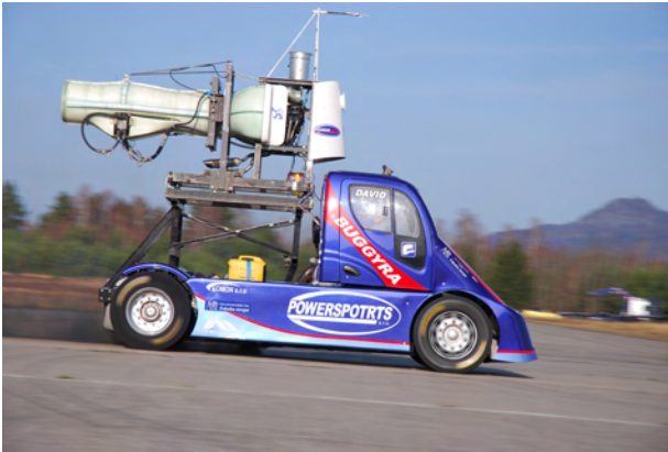
Figure 8: Mobile tests of the propulsion unit with a Buggyra truck.
