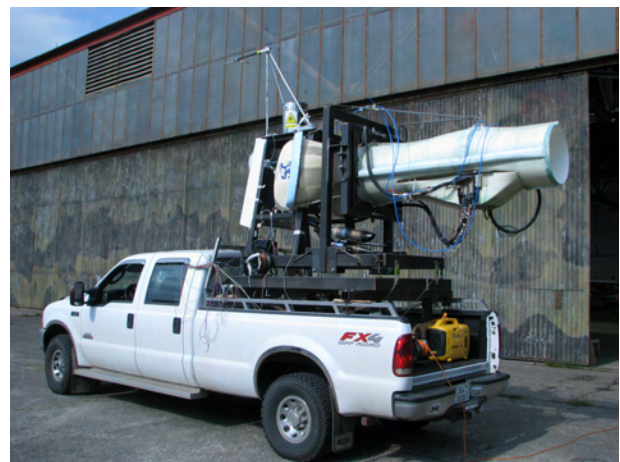
Figure 7: Mobile tests of the propulsion unit with a Ford car.
