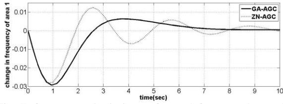
Fig. 7. frequency deviations of area 1 for step change in load (light loading)
