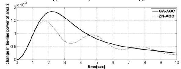
Fig. 16. Tie line power deviations of area 2 for step change in load (light loading)
