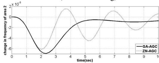
Fig. 10. Frequency deviations of area 2 for step change in load (light loading)
