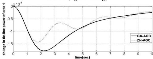
Fig. 11. Tie line power deviations of area 1 for step change in load (heavy loading)
