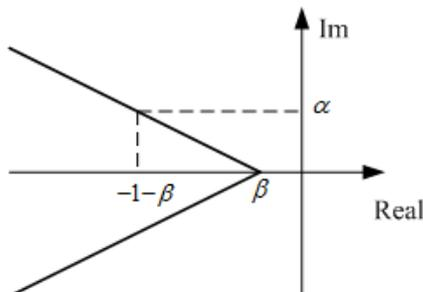
Fig. 3. Wedge shape sector in the complex plane
