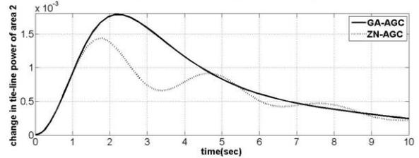
Fig. 14. Tie line power deviations of area 2 for step change in load (heavy loading)
