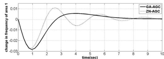
Fig. 5. Frequency deviations of area 1 for step change in load (heavy loading)
