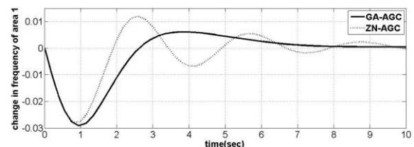
Fig. 6. Frequency deviations of area 1 for step change in load (nominal loading)
