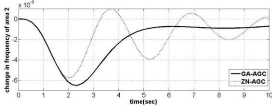
Fig. 8. Frequency deviations of area 2 for step change in load (heavy loading)
