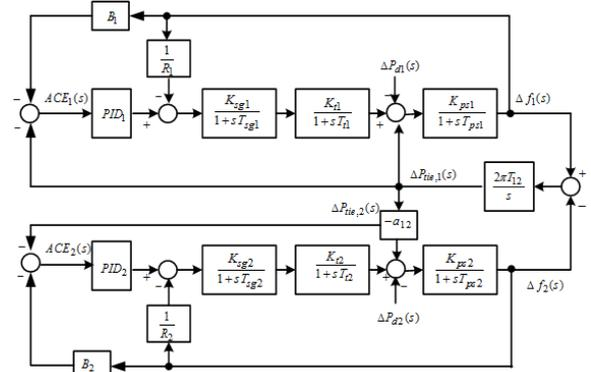
Fig. 2. Transfer function AGC model.
