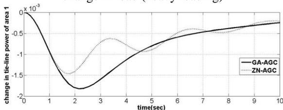
Fig. 12. Tie line power deviations of area 1 for step change in load (nominal loading)
