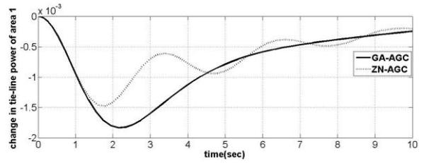
Fig. 13. Tie line power deviations of area 1 for step change in load (light loading)
