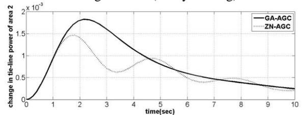
Fig. 15. Tie line power deviations of area 2 for step change in load (nominal loading)
