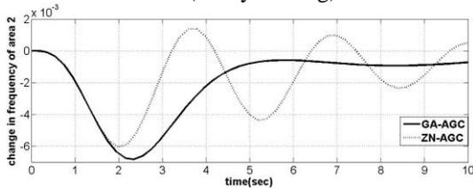
Fig. 9. Frequency deviations of area 2 for step change in load (nominal loading)
