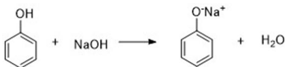
Figure 6. Mechanism of Phenol Converted to Phenoxide Ion
