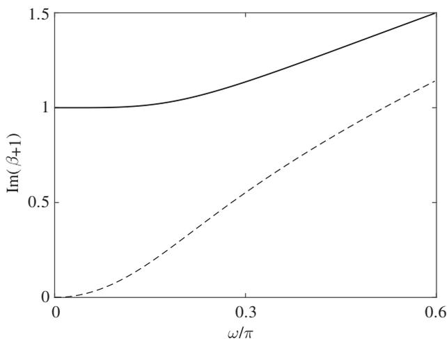
Fig. 1. Imaginary part of complex root  $\beta_{+1}$ , as used by Sergienko (2013) (dashed line) and used here (solid line), given by (17) and (21), respectively, as a function of non-dimensional angular frequency for  $M = 0.0162$ .
