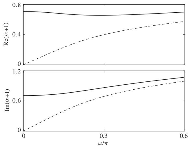
Fig. 2. Real and imaginary parts of complex wavenumber  $\alpha_{+1}$ , as used by Sergienko (2013) (dashed line) and used here (solid line), given by (18) and (23), respectively, as a function of non-dimensional angular frequency for  $M = 0.0162$ .
