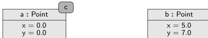
Figure 14: The name c is an example of a reference variable in C++.
