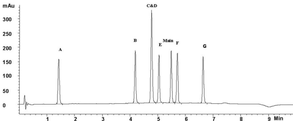
Figure 5. Chromatogram of itraconazole and its impurities developed on RRLLC employing the Agilent Zorbax XDB 1.8  $\mu\text{m}$  column under optimum conditions.
