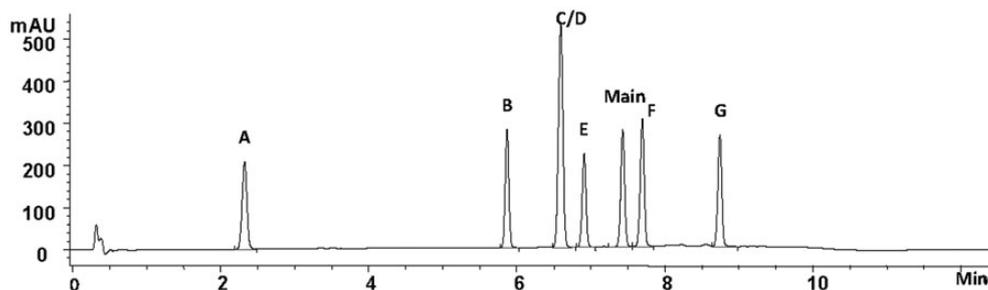
Figure 4. Chromatogram of itraconazole and its related impurities employing an Agilent Zorbax XDB 1.8  $\mu\text{m}$  column on an Agilent 1100 Series, utilizing the optimised gradient method.
