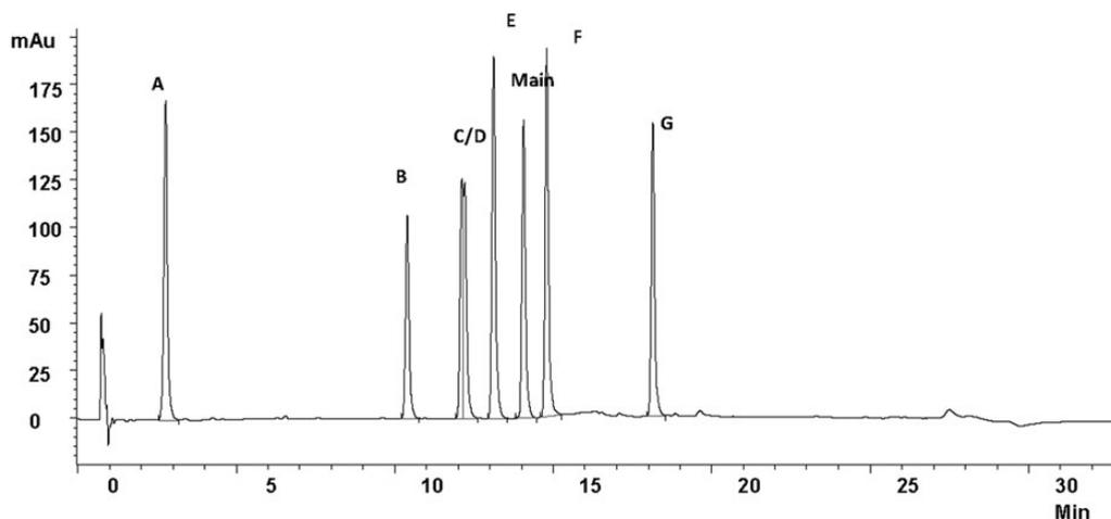
**Figure 2.** Chromatogram for itraconazole and its impurities utilizing the original gradient method.
