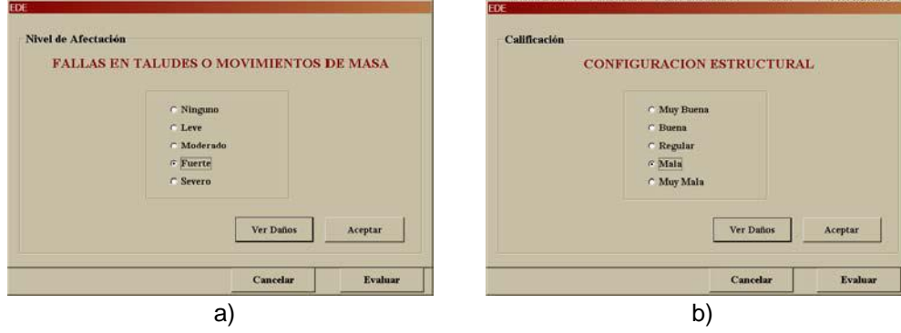
Figure 7: Input of the qualifications for ground conditions and pre-existent conditions. a) Landslides and ground failure, b) Structural configuration.
