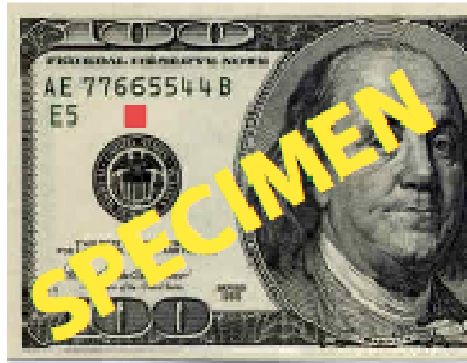
Fig. 1. The red square between the Federal Reserve Bank seal and the serial number on the U.S. $100 bill indicates the ~4 mm 2 region where fluorescence lifetime was collected.
