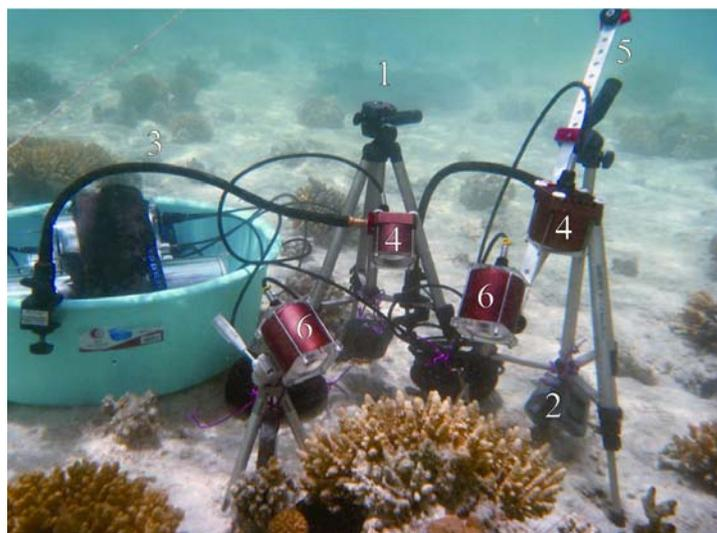
A variety of filters can be used for specific demands. UV- and IR-cut-off filters used during daylight more reliably reproduce color, while an IR-passing filter used during daylight (blocking the visible light), in combination with the IR-light system, provides better insight into the dark regions of highly bright/dark contrasted areas (e.g., interstices of a branching coral).
