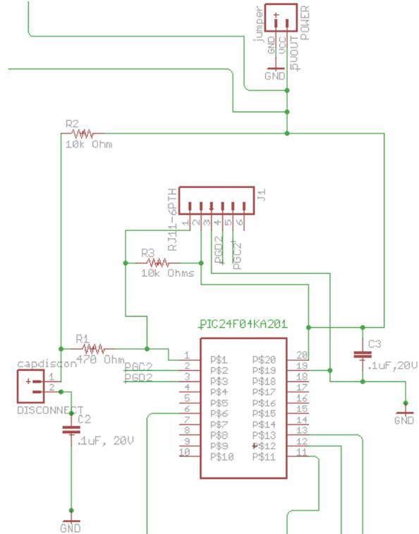
Figure 7 – Power, programming, and required minimum connections for Remote Sensing Unit PCB
