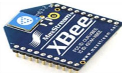
Figure 1 – XBee chip from Sparkfun Electronics
