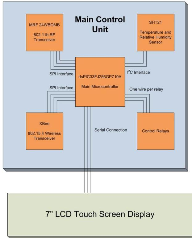
Figure 5 – Main Control Unit Communication Connections
