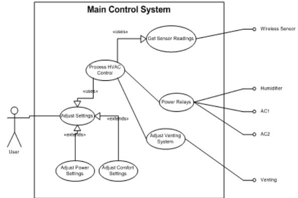
Figure 9 – User Case Diagram for the Main Control Unit
