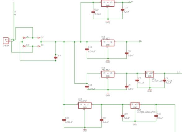
Figure 8 – Power Supply for the Main Control Unit PCB
