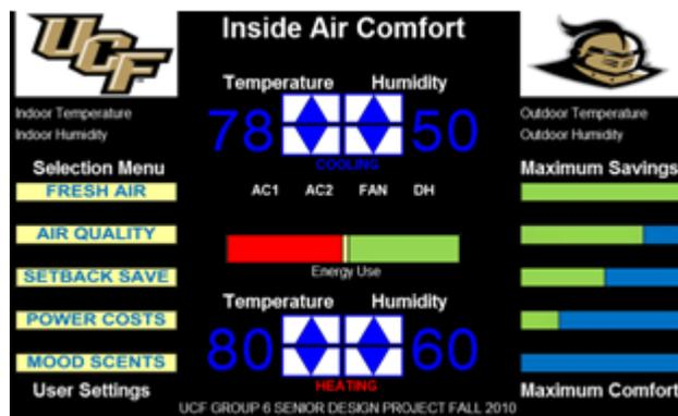
Figure 4 – Main LCD User Interface
