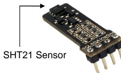
Figure 3 – SHT21 Temperature and Relative Humidity Sensor from Sensirion
