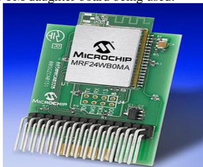
Figure 2 – MRF24WB0MB Wi-Fi RF transceiver with PICtail daughter board from Microchip Direct
