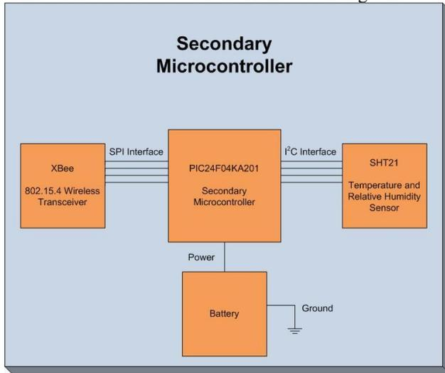
Figure 6 – Remote Sensing Unit Power and Communication Connections
