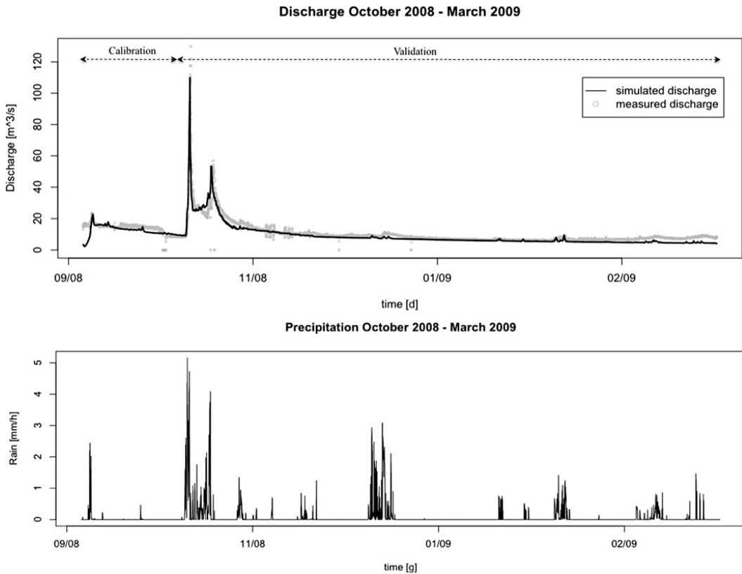
**Fig. 7.** Application of the JGrass-NewAge model for the period 10 January 2008 to 31 March 2009 (winter): the solid curve represents the measured discharge, while the dashed line represents the model simulation data.
