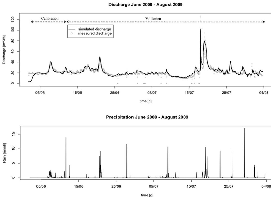
**Fig. 8.** Application of the JGrass-NewAge model for the period 01 June 2009 to 30 July 2009 (summer): the solid curve represents the measured discharge, while the dashed line represents the model simulation data.
