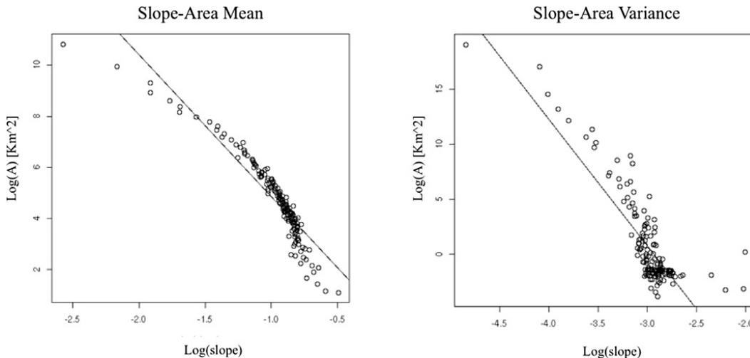
**Fig. 4.** Hillslopes Area – slope relationship in a log-log plot: mean (on the left) and variance (on the right).
