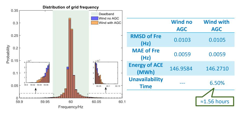
• In the no event case, the wind plant with AGC has few impact on frequency performance of the grid compared with the wind plant without AGC.
