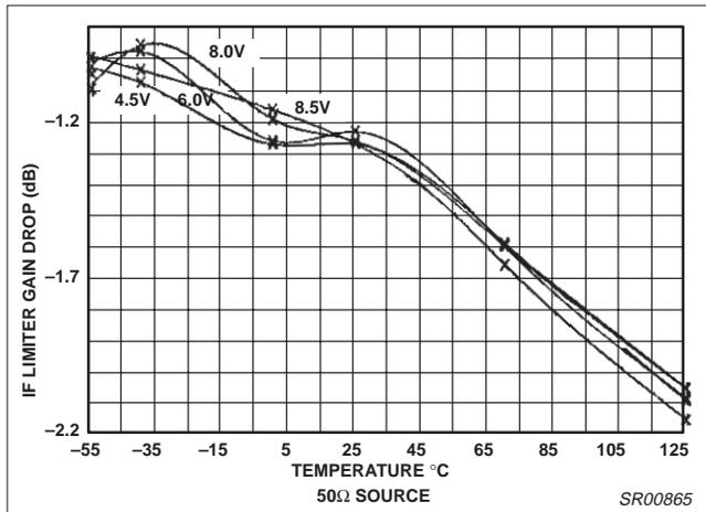
Figure 26. IF Amplifier Gain Drop, 20MHz Response
