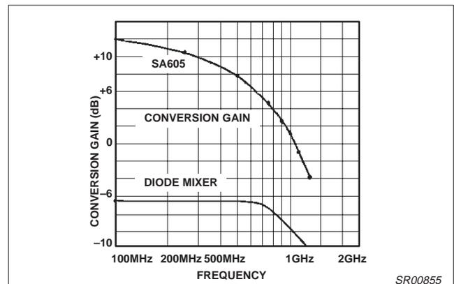
Figure 16. SA605 Conversion Gain vs. Diode Mixer
