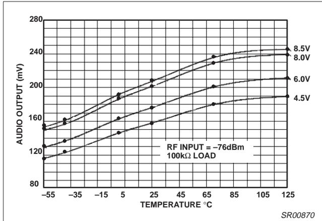
Figure 31. Audio Level vs Temperature and Supply Voltage
