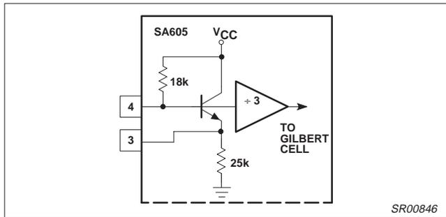
**Figure 7. On-board NPN Transistor for Local Oscillator**
