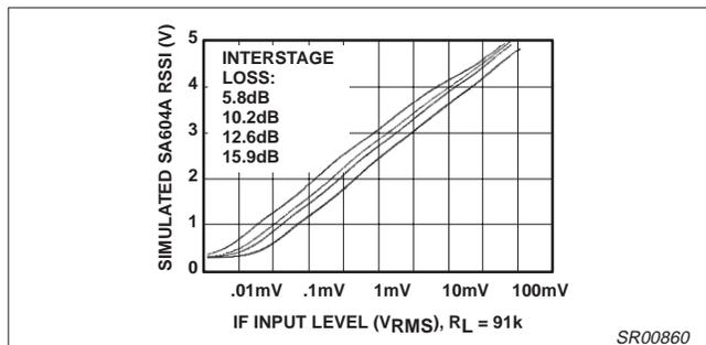
Figure 21. SA604A's RSSI Curve at Different Interstage Losses
