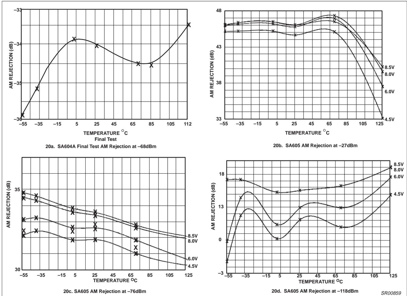
Figure 20. AM Rejection Results at Different Input Levels
