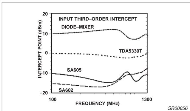
Figure 17. Comparing Different Types of Mixers
