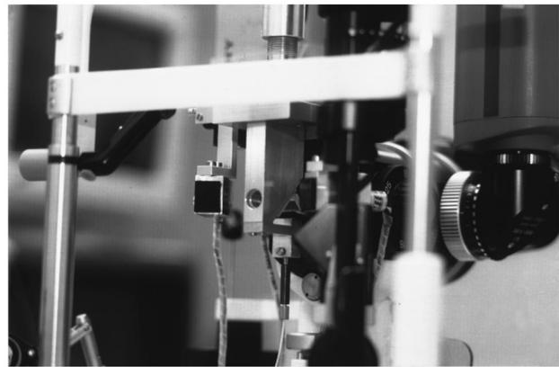
**Fig. 1** OLCR pachometer mounted on a clinical slit lamp (Haag Streit, Switzerland). The LCD and the fixation laser signal are placed in front of the front lens of the slit lamp, allowing the observer to direct the instrument with biomicroscopic stereopsis. The pilot lasers are attached horizontally and converge on the focal distance of the slit lamp, facilitating the alignment of the instrument with the x-y-z control of the slit lamp.
