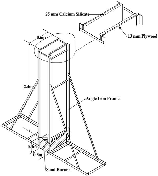
**Fig. 1 Parallel Panel Apparatus**
