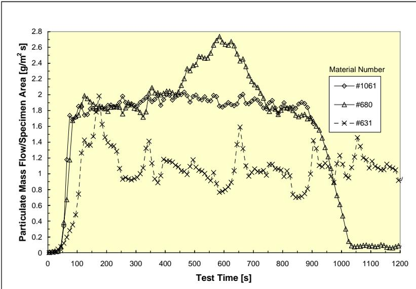
**Fig. 4 Particulate Generation Rate Inferred from Optical Extinction:
