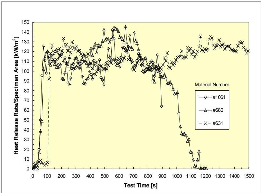
**Fig. 3 Heat Release Rate Measurements in the FPA:
