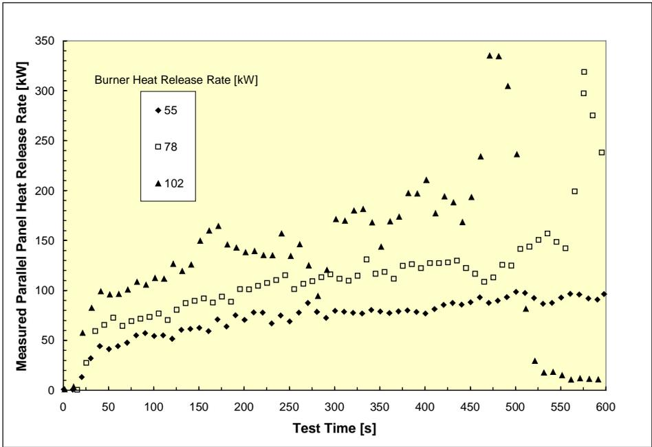
**Fig. 8 Heat Release Rate of Parallel, PVC #680 Panels**
