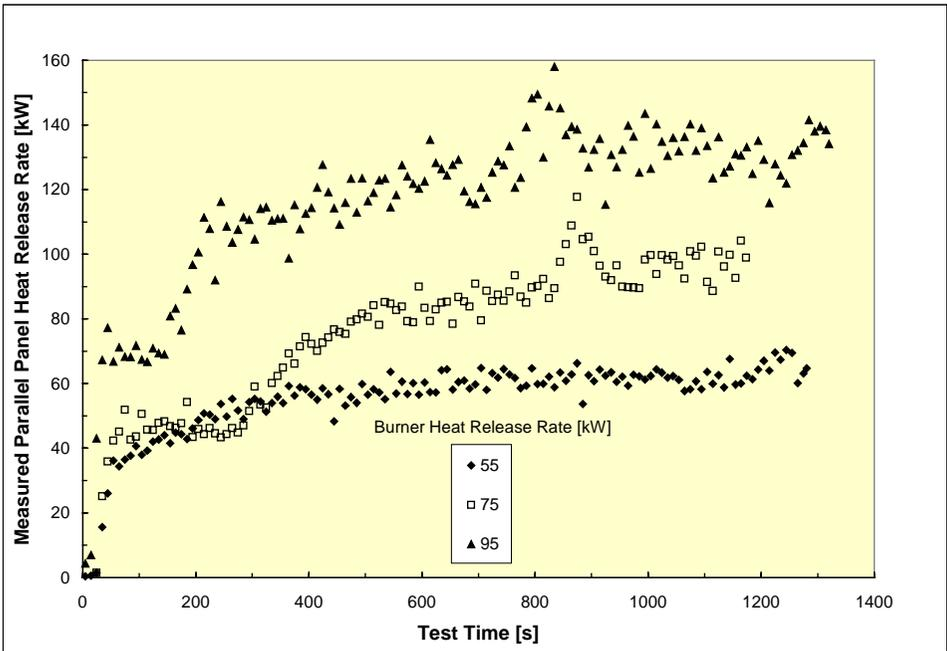
**Fig. 7 Heat Release Rate of Parallel, PVC #1061 Panels**
