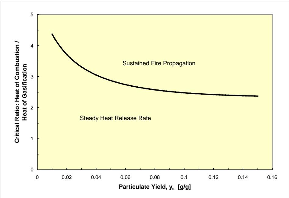
**Fig. 2 Critical Conditions for Sustained Fire Propagation Based on Eq. 9**
