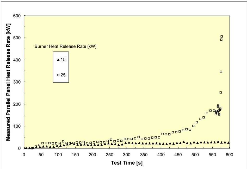
**Fig. 9 Heat Release Rate of Parallel, PP #631 Panels**
