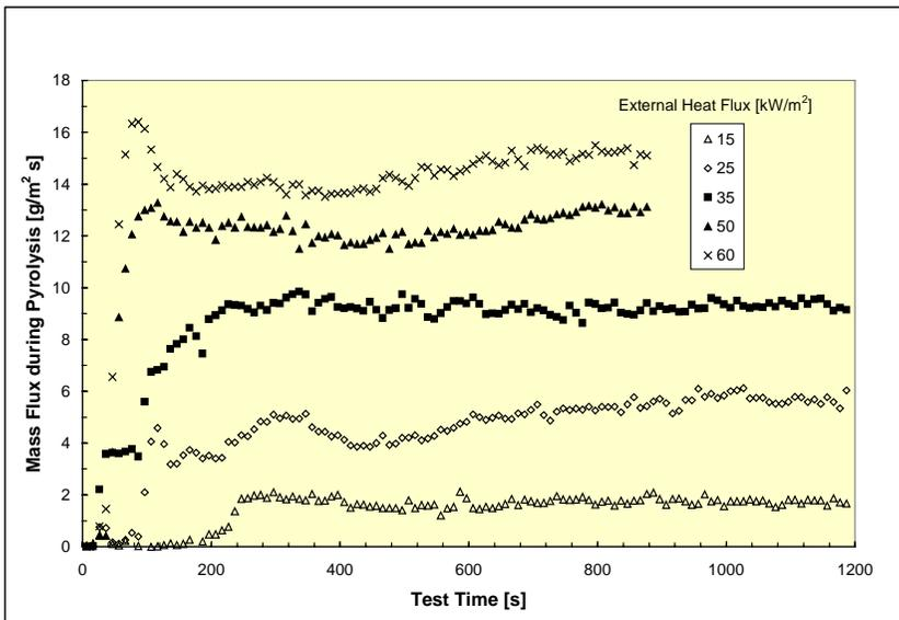
**Fig. 5 FPA Pyrolysis Data for PVC #1061**
