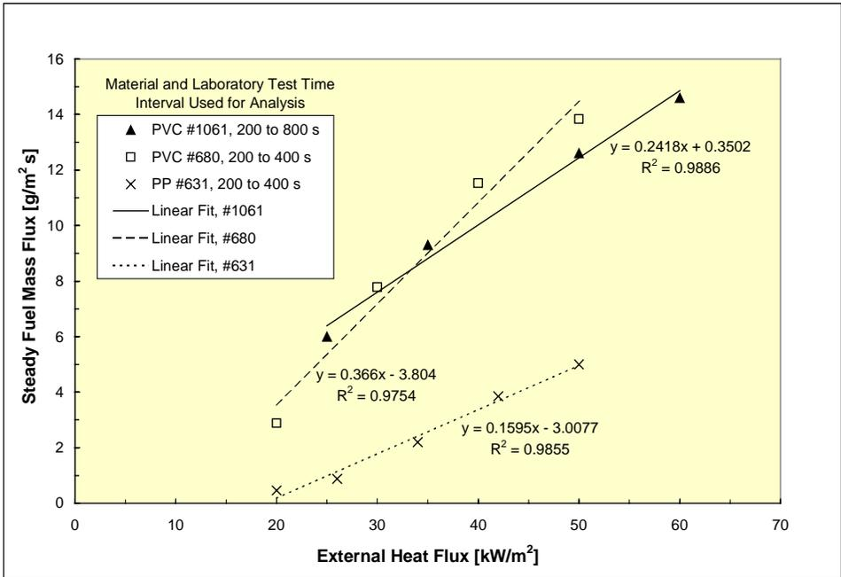
**Fig. 6 Heat of Gasification from Slope of Mass Flux vs. External Heat Flux**
