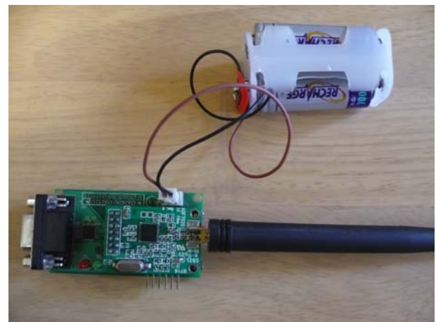
Figure 3. PICSENSE – Sensor node with Battery
