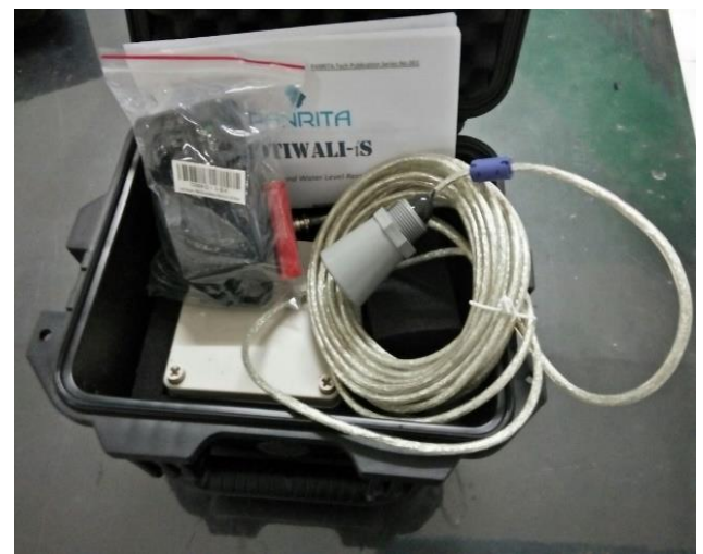
Figure 5. Acoustic Tide Gauge (MOTIWALI).
