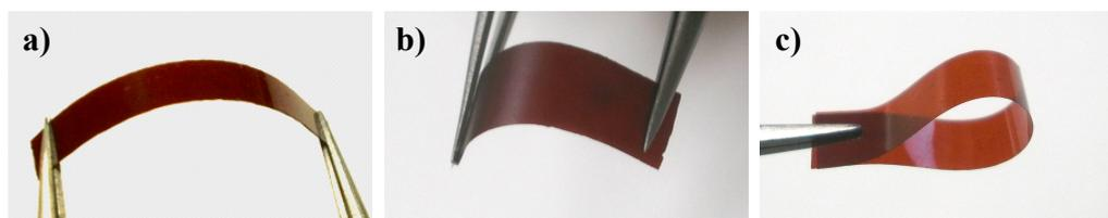
**Figure 10.** Appearance of cured films of PP-4va (a), P(P-4va/MMA) (b), and P(P-4va/BuA) with 33 mol % of BuA composition (c).
