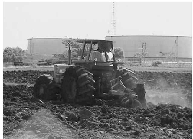
Figure 4. Mechanical aeration of the oily solid in biodegradation process
