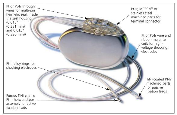
Fig. 2. An implantable cardioverter defibrillator, showing the components that are made from platinum or platinum group metal alloys
