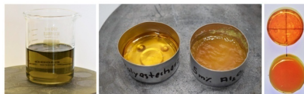
Figure 3. Preparation of the basic mixture (left); hardening of polymer and nanocomposite in tea light shells (center); transparent polymer and opaque nanocomposite (right)
