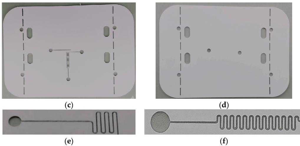
**Figure 6.** Green tapes after the cutting process: (a) Layer 1; (b) Layer 2; (c) Layer 4; (d) Layer 5; (e) Enlarged detail of layer 2; (f) Enlarged detail of layer 4.
