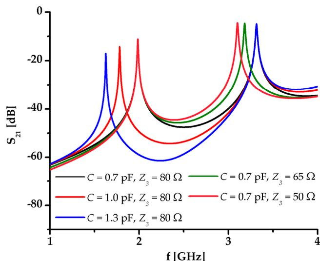
**Figure 2.** Response of the circuit model of the proposed resonator for different values of the capacitance of interdigital capacitor  $C$  and characteristic impedance of the microstrip line whose width is half of the stub  $Z_3$ .
