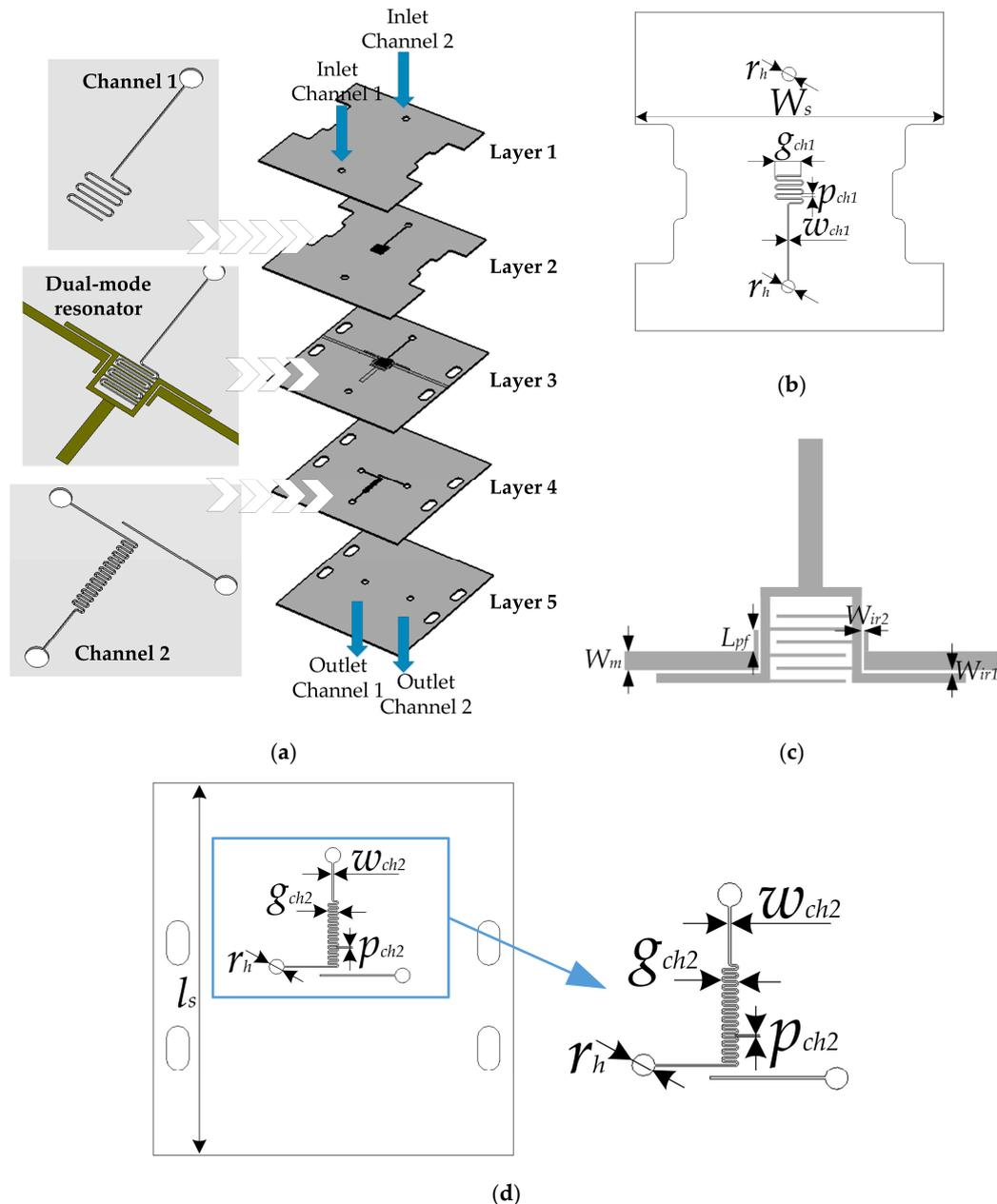
**Figure 3.** (a) 3D layout of the proposed sensor; (b) 2D layout of layer 2; (c) 2D layout of layer 3; (d) 2D layout of layer 4.
