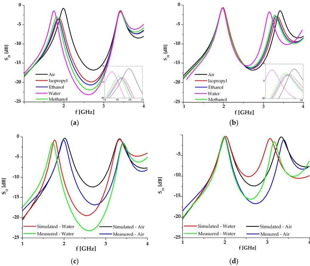
**Figure 10.** (a) Measurement results of the proposed sensor with different fluids placed in channel 1, whilst channel 2 is filled with air; (b) Measurement results of the proposed sensor with different fluids placed in channel 2, whilst channel 1 is filled with air; (c) Comparison of the simulation and measurement results for channel 1; (d) Comparison of the simulation and measurement results for channel 2.
