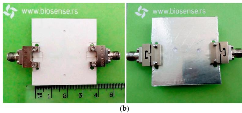
**Figure 8.** (a) The layout of the sensor after the lamination process; (b) The layout of the fabricated sensor—top and bottom view.
