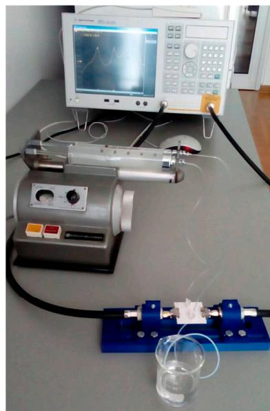
**Figure 9.** Measurement setup for the proposed sensor.
