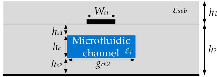
Figure 4. Cross-sectional view of the stub of the proposed resonator.
