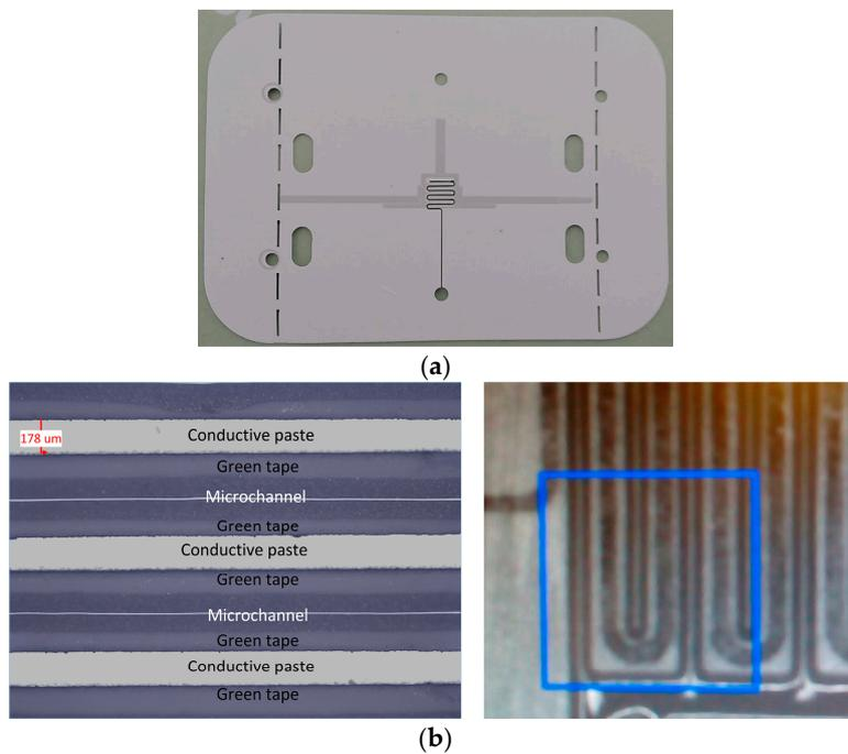
**Figure 7.** (a) Layer 3 after the cutting and screen printing processes; (b) Details of the interdigital capacitor with the meandered microfluidic channel in layer 3.
