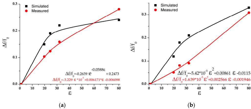
**Figure 11.** Frequency change ( $\Delta f/f_0$ ) versus the change of fluid permittivity for: (a) Channel 1; (b) Channel 2.
