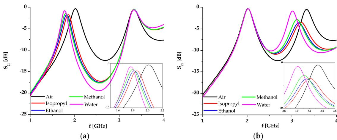
**Figure 5.** (a) Simulation results of the proposed sensor with different fluids placed in channel 1, whilst channel 2 is filled with air; (b) Simulation results of the proposed sensor with different fluids placed in channel 2, whilst channel 1 is filled with air.
