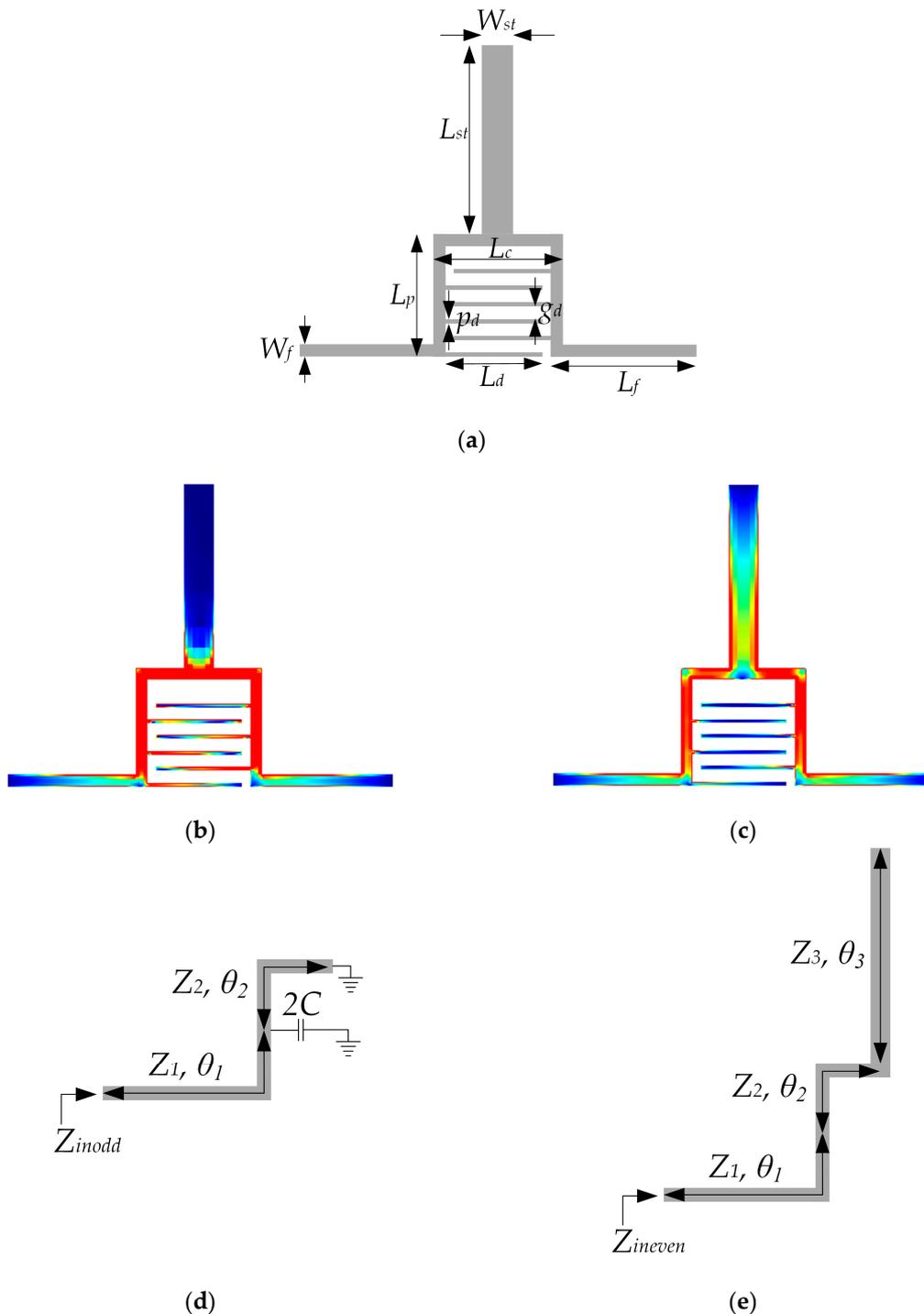
**Figure 1.** (a) Configuration of the proposed dual-mode resonator; (b) Current distribution for the odd mode; (c) Current distribution for the even mode; (d) Odd-mode equivalent circuit; (e) Even-mode equivalent circuit.
