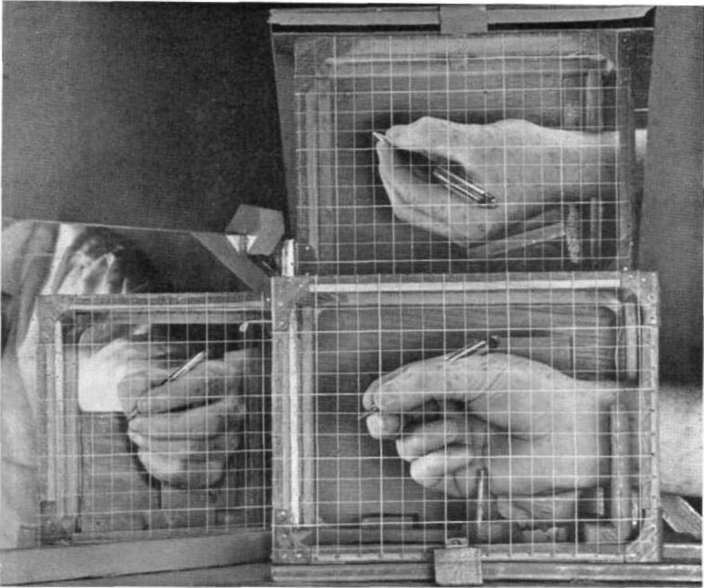
Fig. 8. Cage for observing hand prehension patterns in three dimensions simultaneously. The grasp shown is the typical palmar prehension of the three-jaw-chuck variety. *Courtesy University of California at Los Angeles.*
