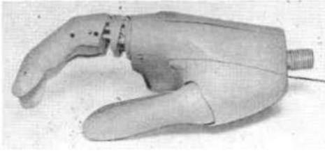
Fig. 6. Experimental hand with palm section of monocoque construction. The finger design shown, also experimental, is one of many tested. See Figures 9 and 10. *Courtesy Army Prosthetics Research Laboratory.*
