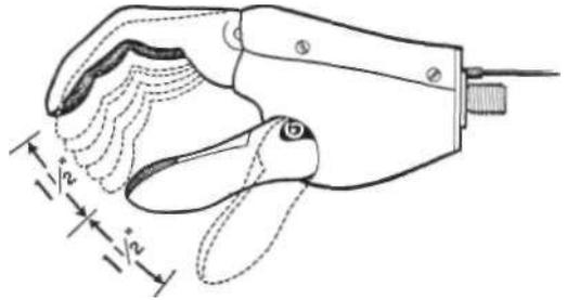
Fig. 11. The two-position thumb, set manually from either position to the other by application of pressure on the dorsal side. Inner position provides for objects up to 1-1/2 in. Outer position accommodates objects between 1-1/2 and 3 in.
