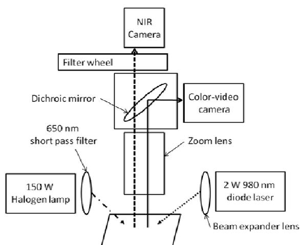
**Fig. S5** Outline of real-time multiplexed NIR imaging setup.
