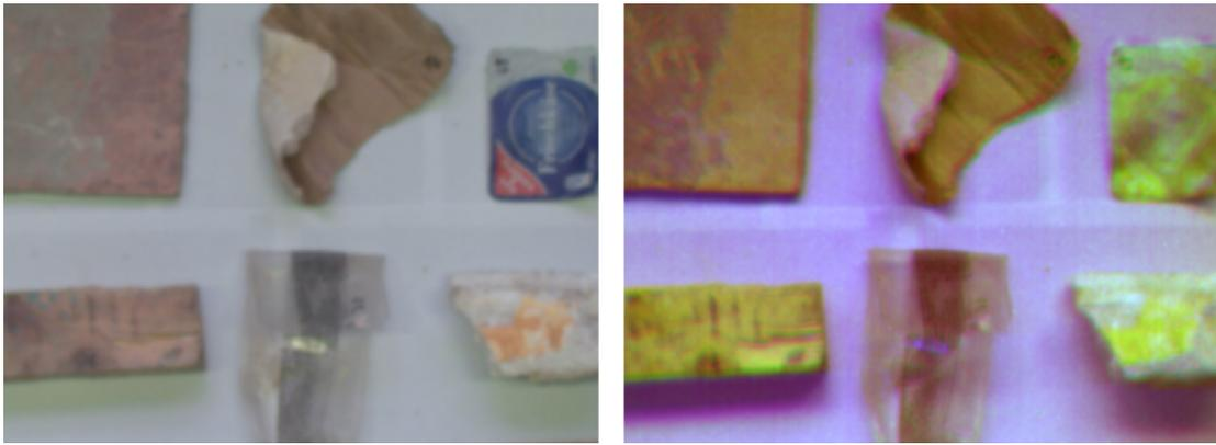
Figure 4: Left: RGB image of six sample pieces in the visual spectrum. Right: false-color image with the spectra around 880 nm, 1300 nm, and 395 nm (Kaßmann et al., 2021b, under CC-BY 4.0).
