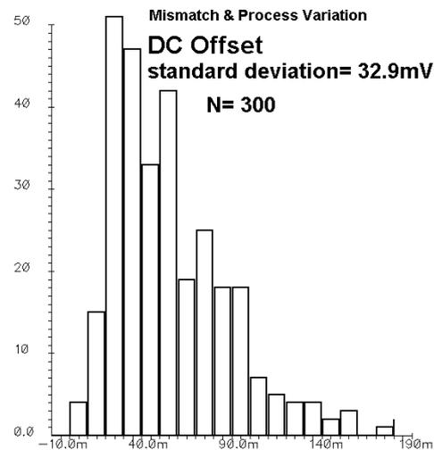
**Figure 5 Results of the corresponding mismatch and process simulations**
