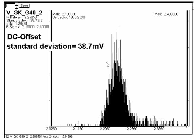
**Figure 4 Measured offset spread of a complex amplifier stage**
