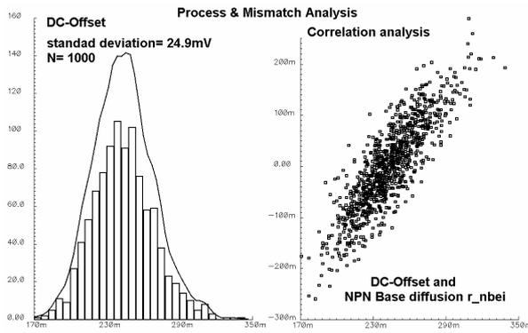
**Figure 2 DC offset spread and correlation with NPN base doping  $r_{nbei}$**
