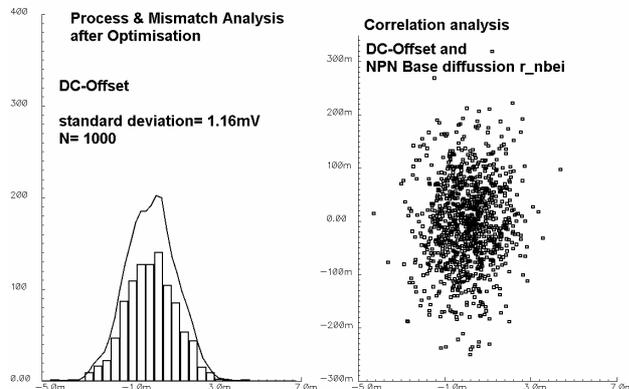
**Figure 3 After the optimization the DC offset spread is minimized and its dependence on NPN base doping  $r_{nbei}$  disappeared**
