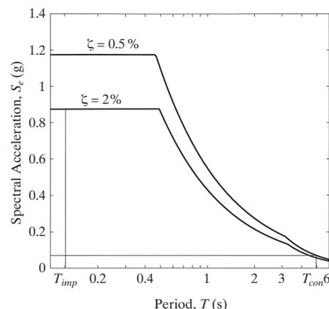
Fig. 7: Elastic design response spectra for 0.5% and 2% damping
