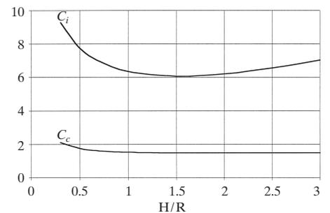
Fig. 4: Impulsive and convective coefficients  $C_i$  and  $C_c$
