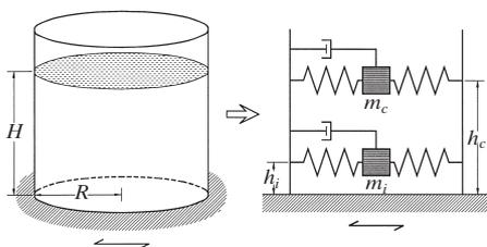
Fig. 3: Liquid-filled tank modelled by generalised single-degree-of-freedom systems
