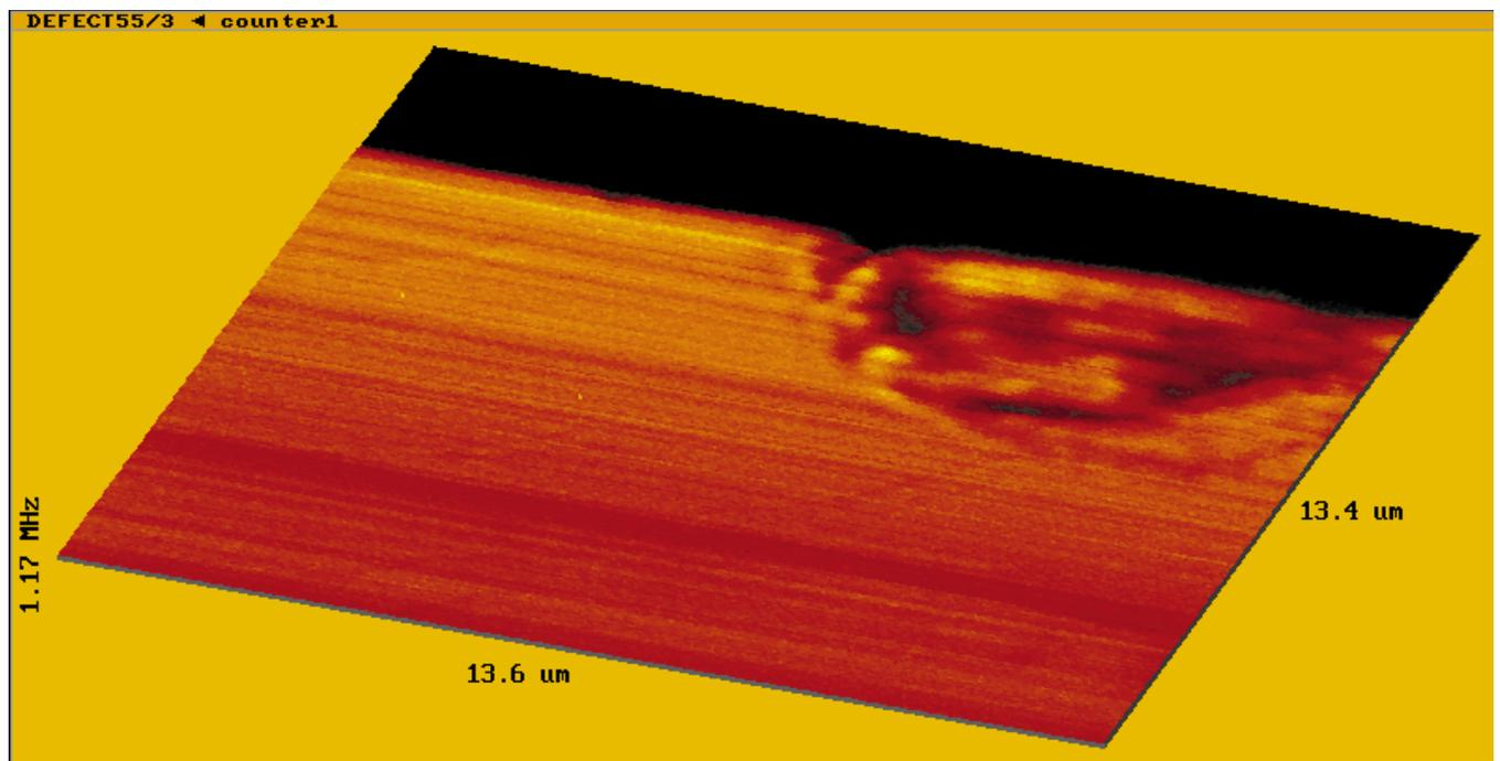
Fig. 2. (A) AFM and (B) transmission NSOM of a chrome defect ablated with an ArF excimer laser.
