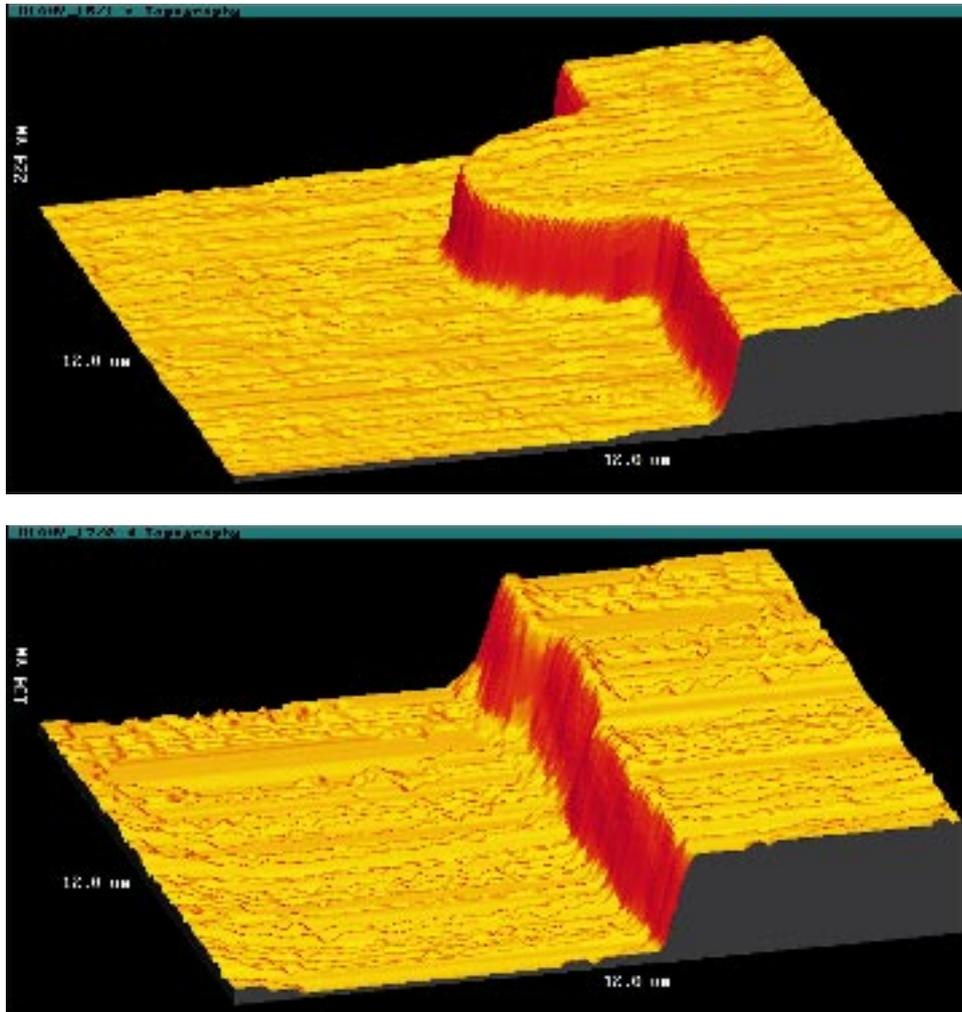
Fig. 4. (A) AFM image of a programmed defect prior to repair. (B) AFM image of the same region after repair.
