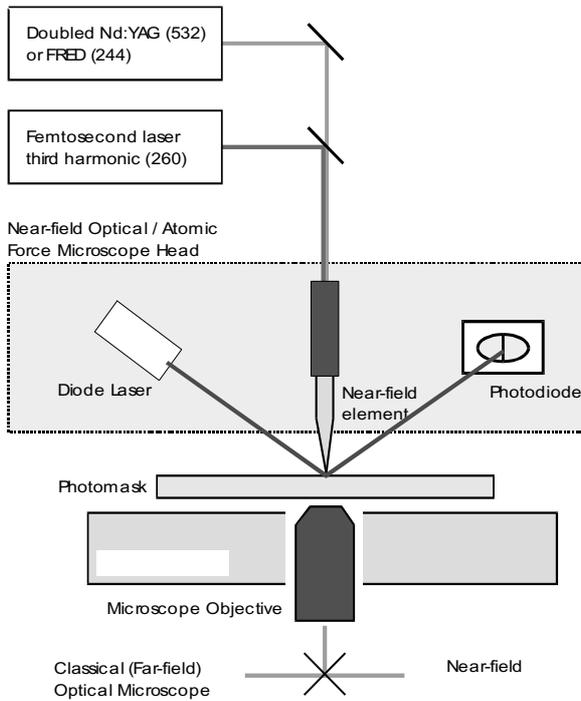
Fig. 1. Schematic layout of the MR-100 near-field system.
