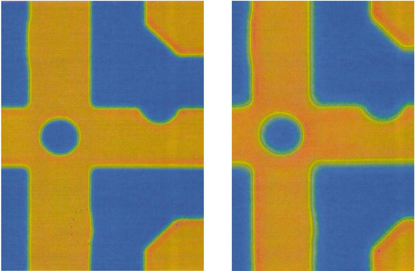
Fig. 5. Aerial imaging data (AIMS) at 248 nm of two repaired defects. (A) Image best focus, (B) plus 1  $\mu\text{m}$  defocus.
