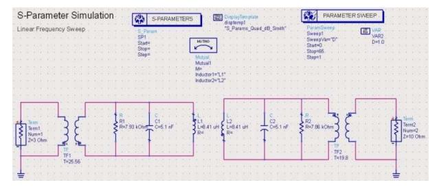
Fig. 3: Schematic diagram for S-parameter simulation using ADS
