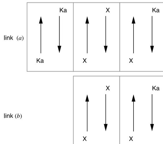
**Figure 3.** The combinations of coherent links to be considered. (a) X and Ka up and down, with an additional Ka down-locked to the X phase on board (three observables). (b). X up and down, Ka down locked to the X phase on board (two observables). Combination (a) is the prime operation mode of the experiment, but will be available for only  $\frac{1}{3}$  of the time, or for more than  $\frac{2}{3}$  of the time if the Sardinia antenna will be available. Combination (b) is a backup.
