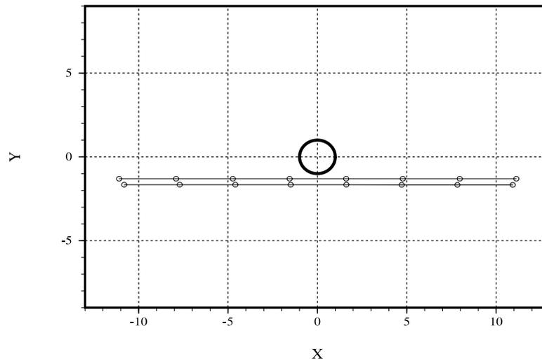
**Figure 4.** The trajectory of Cassini projected in the plane passing through the Sun and normal to the Earth–Sun direction, as seen from an observer on the Earth, during the conjunction experiments of 2002 (top) and 2003 (bottom). The ticks are separated by 1 day.
