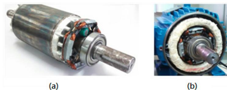
**Figure 9.** System coupled to the rotor. (a) Outside the stator; (b) inside the stator.
