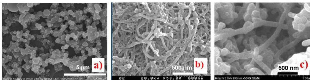
**Figure 2.** TEM images of SWNTs (a); PPy/SWNTs nanocomposites (b) and PPy layer/shell on the surface of amorphous carbon and out of SWNTs bundle core (c).
