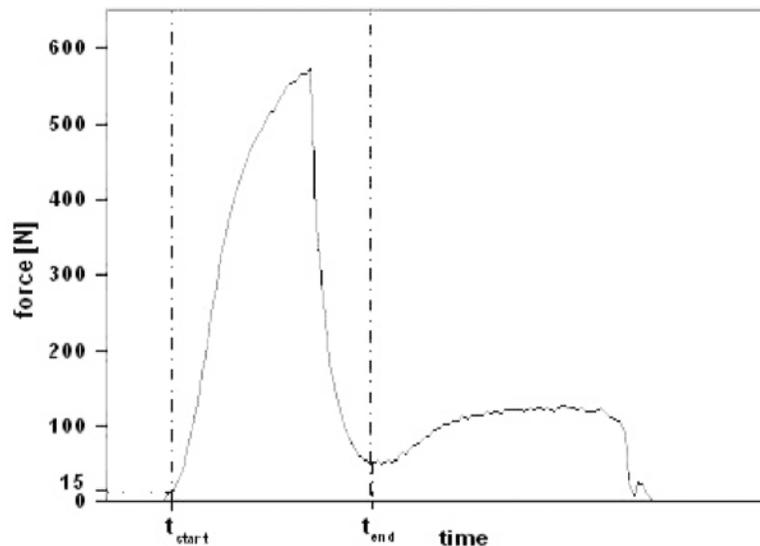
**Figure 1** — Determination of the impact phase from  $t_{\text{start}}$  to  $t_{\text{end}}$ . The impact phase started when the reaction force exceeded 15 N and ended at the first local minimum after the force maximum.
