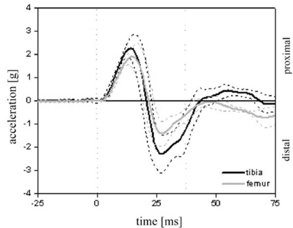
**Figure 4** — Representative acceleration time histories for the tibial and femoral acceleration ( $ACC_{\text{tib}}$ ,  $ACC_{\text{fem}}$ ). Mean and standard deviation curves for one subject at 20° knee angle at the 30% contraction level.
