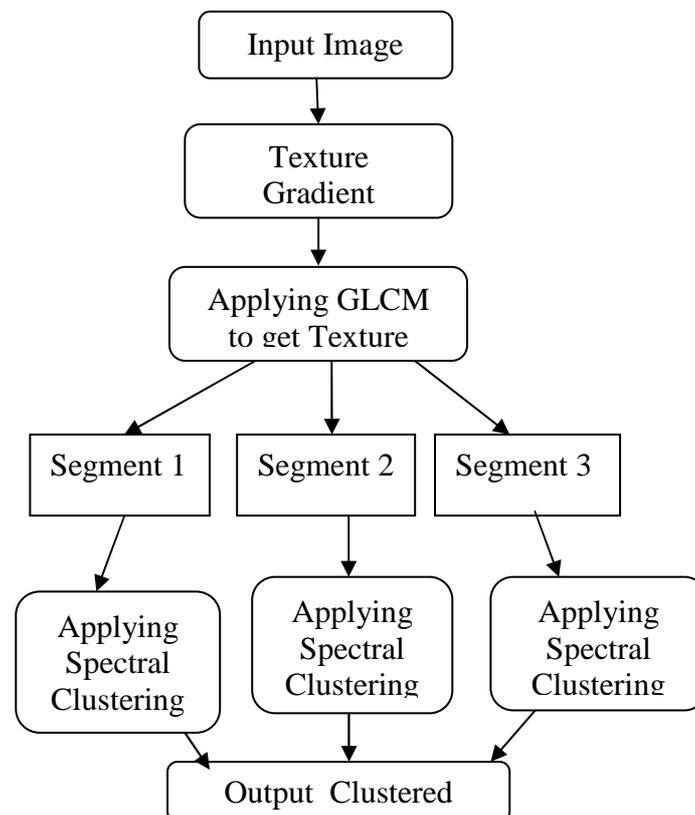
Figure 3. Flow chart for image segmentation using Spectral Clustering.
