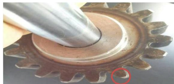
Figure 2. The gear with faulty tooth.
