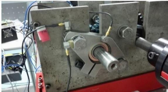
Figure 3. Accelerometers location on the bearing housing.
