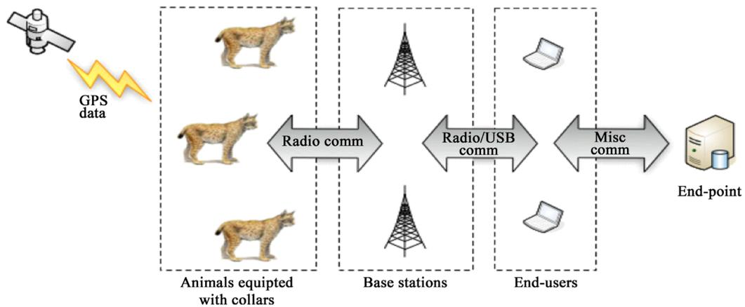
Figure 2. Lynx net system architecture [4].
