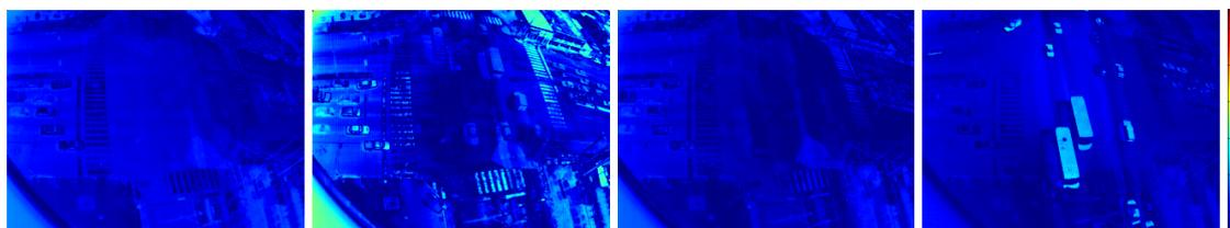
**Figure 11.** The enhancement of binary motion maps. The motion objects are better defined, and the noise effects are discarded. In (a) the original frames; in (b) the estimation of  $B(\mathbf{x})$ , and in (c) the enhancement map  $\tilde{B}(\mathbf{x})$ .
