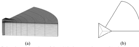
Fig.1 (a) Typical finite element meshes of the 1/6 indenter and nacre. (b) The geometrical relationship between Berkovich indenter and the indented section.
