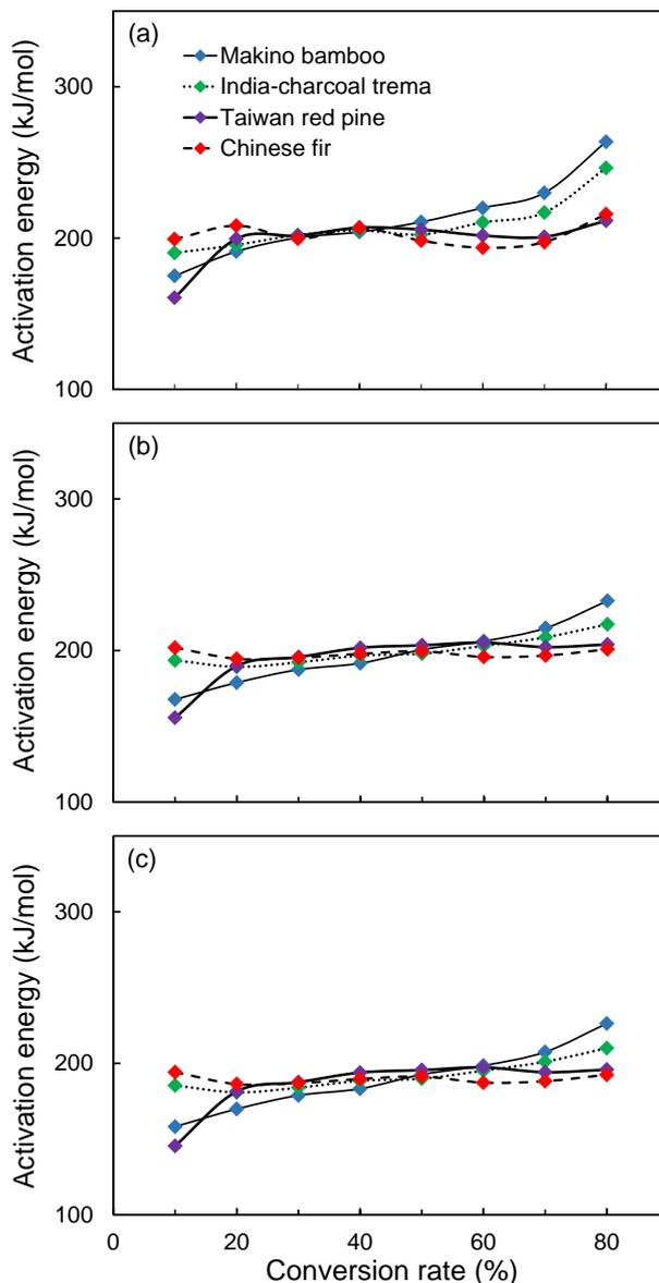
**Figure 6.** A comparison of apparent activation energies as a function of decomposition conversion rate ( $\alpha$ ) for various lignocellulosic fibers calculated by the Friedman method (a); Flynn-Wall-Ozawa method (b); and modified Coats-Redfern method (c).
