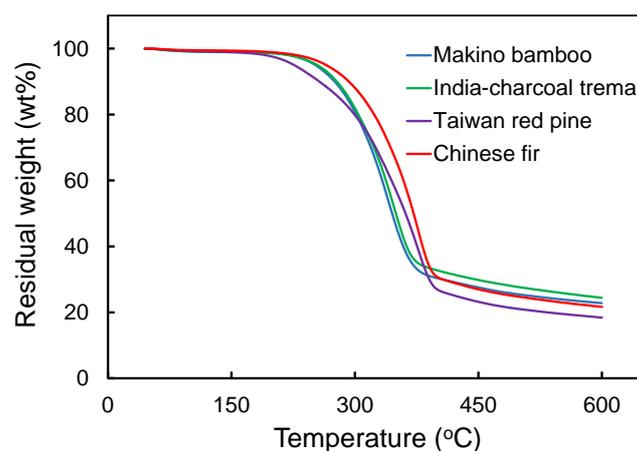
**Figure 4.** Thermogravimetric analysis of various lignocellulosic materials at a heating rate of 20 °C/min.
