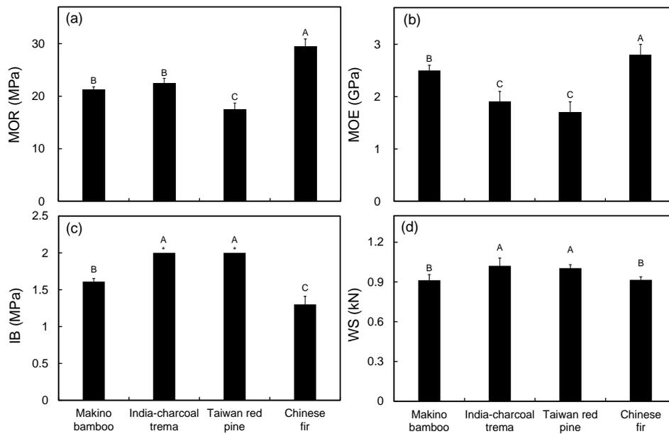
**Figure 3.** The MOR (a); MOE (b); internal bond strength (IB) (c); and wood screw holding strength (WS) (d) of WPCs made with different lignocellulosic fibers. \*: IB over the test limitation (2 MPa). Values are the mean  $\pm$  SD ( $n = 5$ ). Different letters indicate significant differences among groups ( $p < 0.05$ ).
