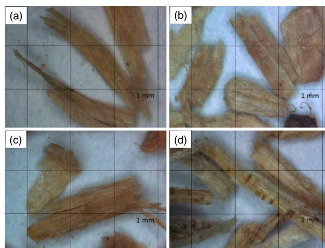
**Figure 1.** Micrographs of different lignocellulosic fibers: (a) makino bamboo; (b) India-charcoal trema; (c) Taiwan red pine; and (d) Chinese fir.
