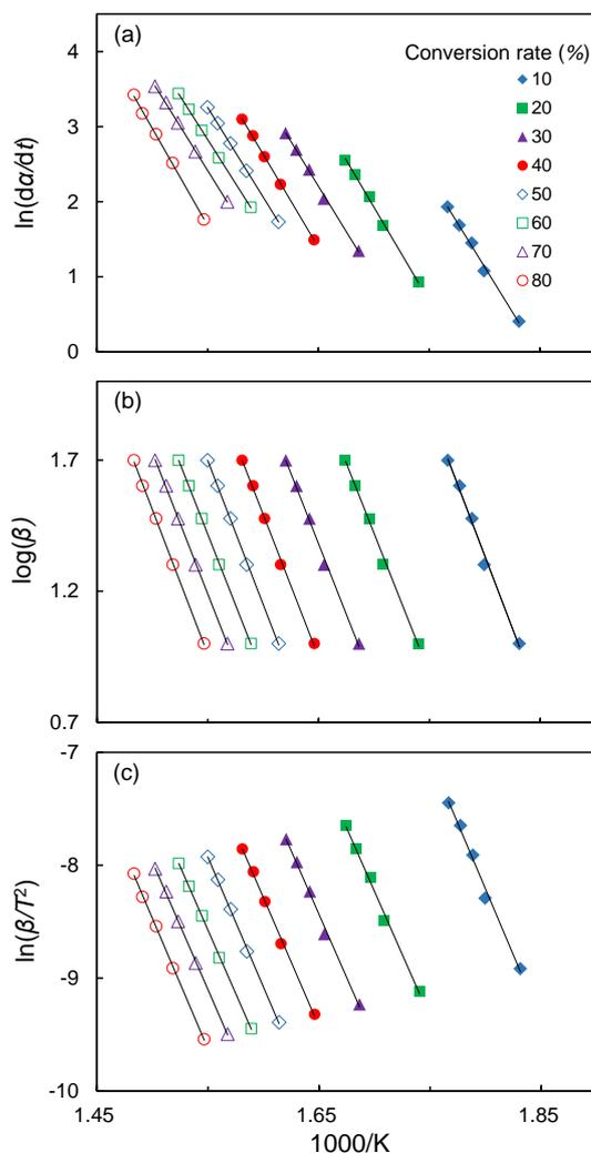
**Figure 5.** Typical isoconversional plots using the Friedman method (a); Flynn-Wall-Ozawa method (b); and Modified Coats-Redfern method (c) for Chinese fir.
