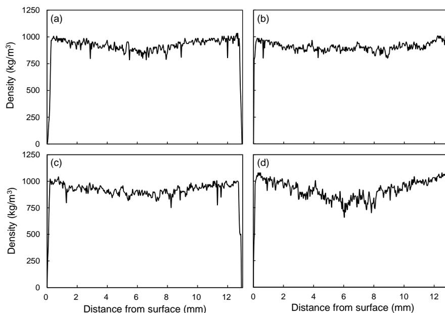
**Figure 2.** The vertical density profiles of WPCs made with makino bamboo (a); India-charcoal trema (b); Taiwan red pine (c); and Chinese fir (d).
