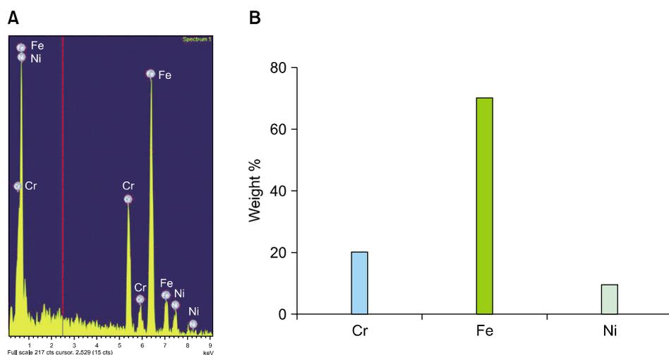
**Fig. 2.** Energy-dispersive X-ray spectroscopy (EDS) imaging: (A) Nickel and chromium components at the skin-contacting parts of the spectacle frames. (B) The mean nickel content (weight, %) was  $15.7 \pm 5.5$ , and the mean chromium content was  $20.3 \pm 3.4$  at the skin-contacting part of the spectacle frames.
