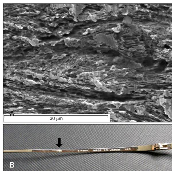
**Fig. 1.** (A) Scratches on the skin-contacting parts of the spectacle frames analyzed by scanning electron microscopy (SEM). (B) Black arrow indicates the skin-contacting part.
