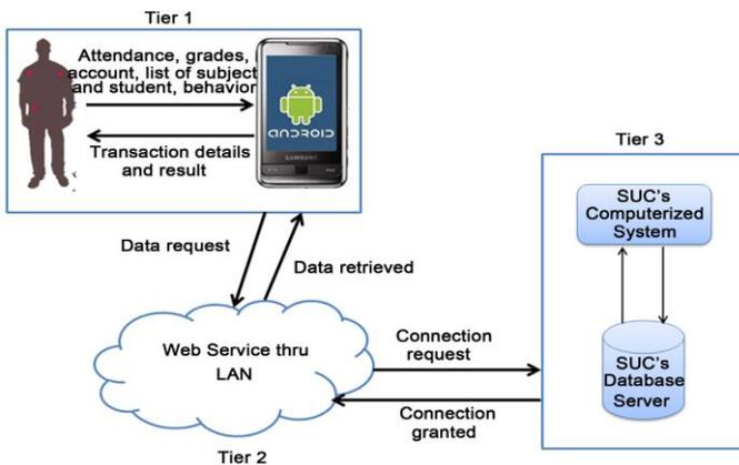
Figure 1. System Architecture of Android Based Class Record System [2]
