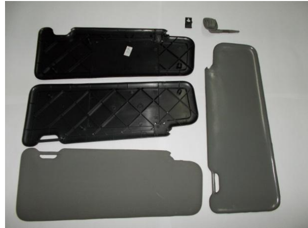
Fig. 3. Component elements of sun visor
