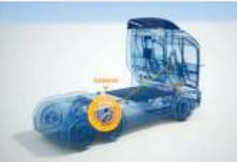
Sensors in key areas of the truck identify and transmit data on material degradation or damages. Analytics can predict asset failures and automatically schedule maintenance checks when needed (See [MoDE](#)).
