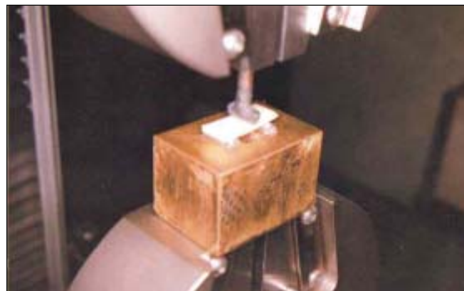
Figure 5: Specimen mounted on Instron testing machine
