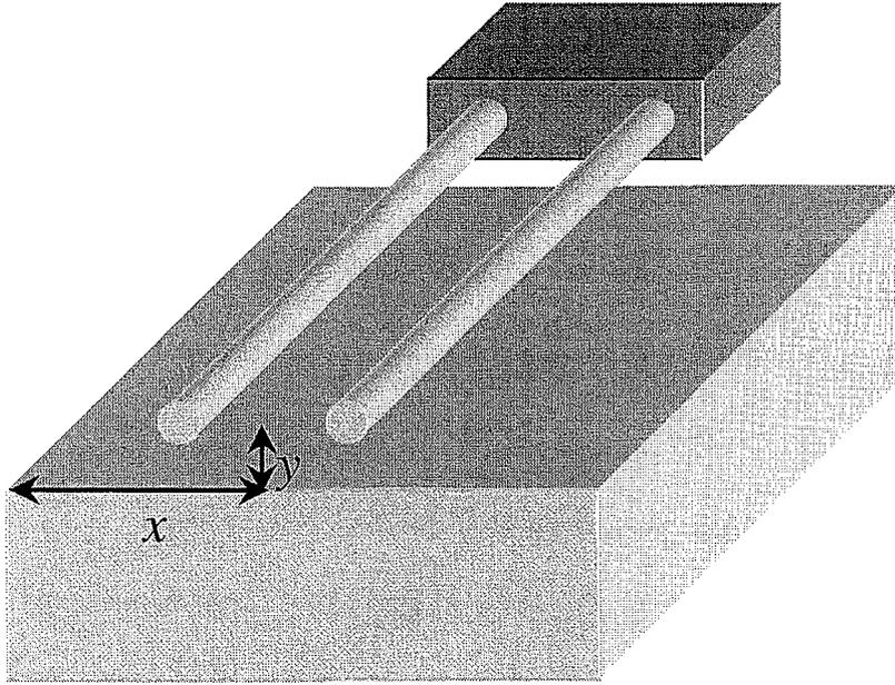
**Fig. 2. Position of transmission line and phantom dielectric body.**
