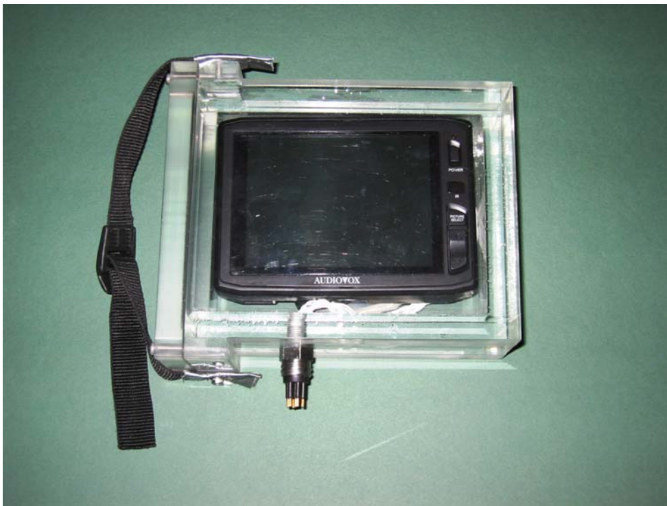
Figure A1: LCD Monitor in pressure proof underwater housing
