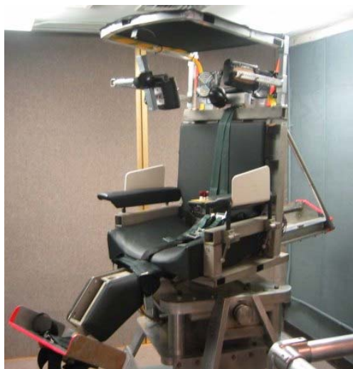
Figure 2. Rotating chair, showing adjustable head stops and visual canopy (being closed).
