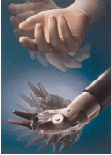
Figure 8. a) The Endo Wrist developed by Intuitive Surgical Systems for minimally invasive cardiac procedures and b) The Slave robotic system with various surgical tools for performing the surgery. (Figures 8(a) and 8(b) From “The heart of microsurgery”, J. K. Salisbury, Jr. In Mechanical Engineering, American Society of Mechanical Engineers , 1998.
